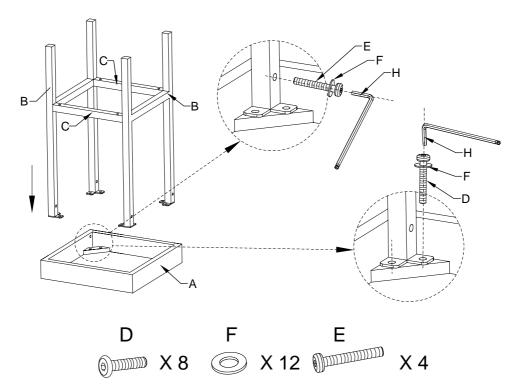
Step 3. Using bolts (D), and washers (F) attach stretchers (C) to foot panels (B).
