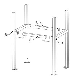
Step 2. Lay seat (A) down on a flat surface.Attach assmbled parts B, C to the seat (A) using bolts (D), washers (F), allen key (H) in vertical direction. Cross direction by using bolts (E),washers (F), allen key (H). NOTE: Do not fully tighten bolt until all bolts are in place.
